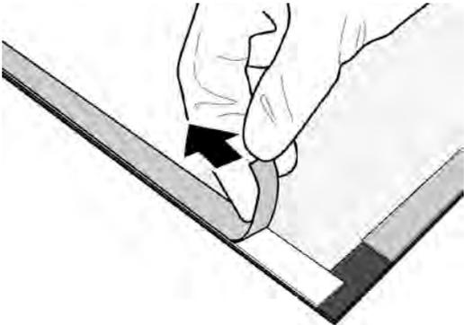
6. The picture below shows the tear off tape of the 4 metal strips.
