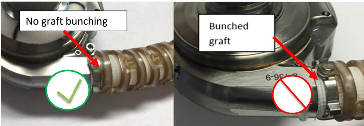
6. Verify that the clamp screw is on the outflow conduit and attached to the graft clamp. If the clamp screw is completely removed or if it falls out, be sure to re-insert it correctly as the clamp has threads on only one side.
