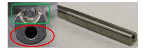
Example of the unfinished dual carrier (two separate angles). The highlighted oval area in red (or bottom) is not machined/milled out. It should be similar to the opposing top side highlighted in green rectangle area.
