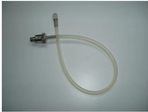
Figure 3: Test all adapters with the laser imprint EUS-XMB. Test the complete adapter. Do not dismantle the adapters.
