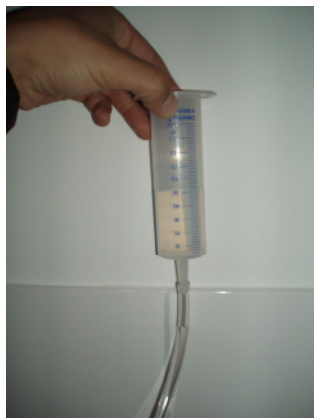
Figure 5: Remove the piston of the syringe and fill in 50 ml of water
