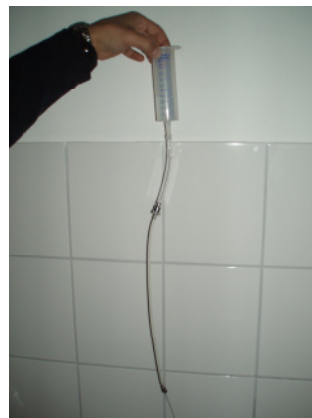
Figure 6: Water will flow through the adapter. By gravity 50 ml will flow out within a maximum of 60 seconds. If no water flows through the adapter, inform Olympus
