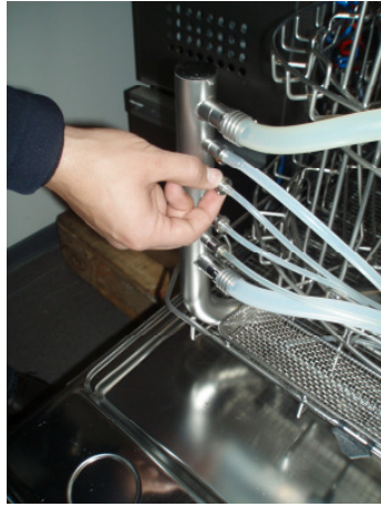
Figure 1: Disconnect the adapter from ETD2 / mini ETD. Perform the test outside of ETD machine by using a syringe.
