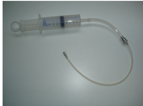
Figure 4: Connect the syringe via a silicone tube to the adapter, while applying the same flow direction as in the ETD machine.
