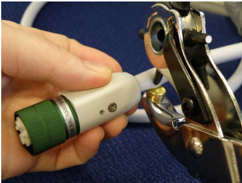
Picture 2. How to make the hole?
