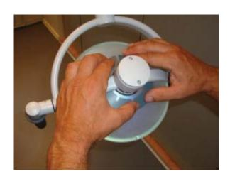
5. Pull back the one tab to partially remove the protective paper a little over halfway; position the foil under the arc again and press it into place while removing the rest of the protective paper from the opposite side.
