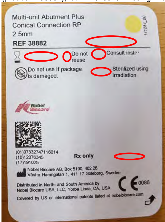
Figure 2. The photo shows the incorrect product label for the Multi-unit abutment Plus CC RP 2.5mm (product # 38882), lot # 12076345. Missing information highlighted in red.
