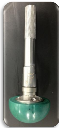
Figure 4: 36mm and 42mm diameter impaction assemblies.
