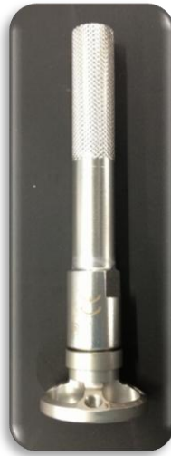
Figure 2: Assembly of drill guide to Handle.
