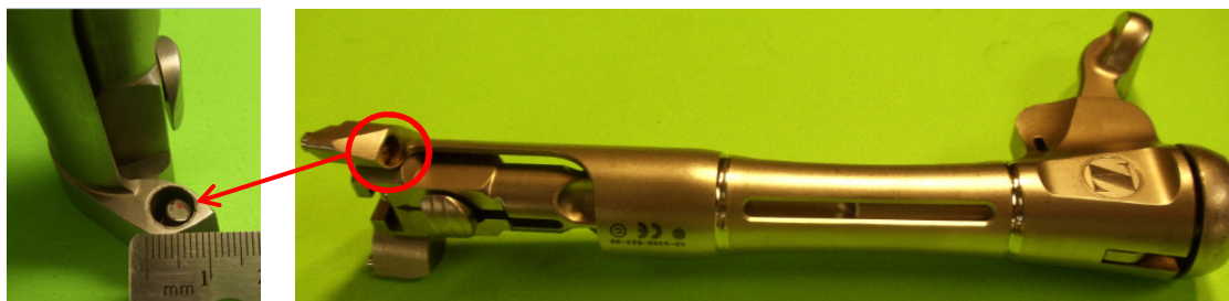
Right: Persona Cemented Tibial Broach Inserter/Extractor Handle with disassociated magnet cover Left: View of guide with disassociated magnet cover
