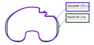
Figure 1: Drawing of Tibia Trial Plateaus T3+ and T4
