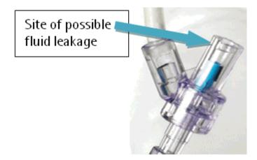
The silicone disc is not returning into closed position after disconnection of male Luer cone counterparts. Valves, unused or fully connected do not show this defect.
