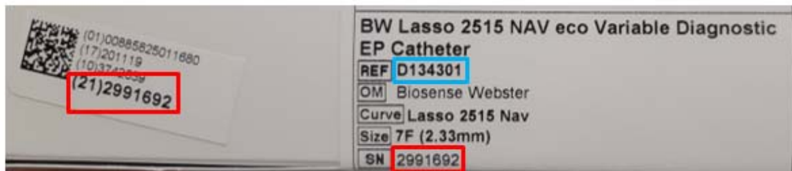
Figure 2: Labels on top edge of box. Device serial number is outlined in red and catalog number is outlined in blue.
