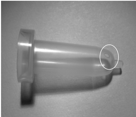
Figure 1: Location of HM Vessel Defect, if present
