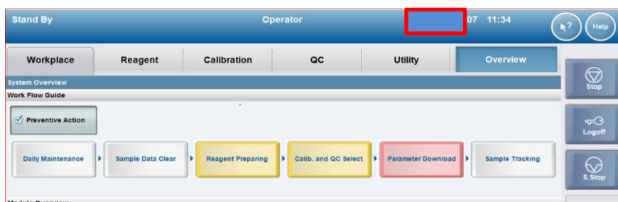
Figure 1: Date (in the red box) not displayed in the Status Line of the User Interface
