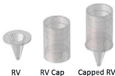
Figure 1. Excerpt from Alinity m Operations Manual, 54-605001/R10, depicts the RV, RV Cap, RV and RV Cap (RV assembly).
