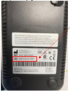
The instrument Serial Number can be verified on the label on the underside of the instrument
