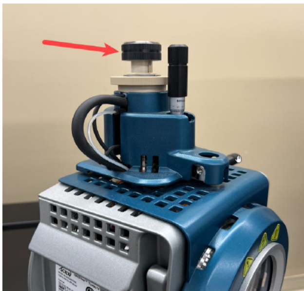
Figure 2: Replacement nut featuring a groove is mounted on top of the probe assembly.
