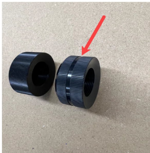
Figure 1: The groove on the replacement nut (right) that distinguishes it from the original nut (left).
