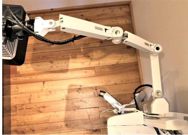
Figure 2: Please avoid this unfavorable positioning of the arms, as when adjusting the height of the camera in this position, high leverage forces act on the first arm element.
