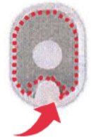
Gel almost completely missing
