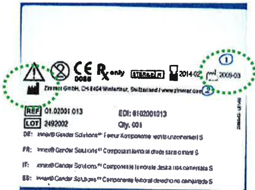
Figure 1: Example of a representative product label providing (1) is the manufacturing date (“white” production plant symbol), and (2) the manufacturing site (“dark” production plant symbol)
