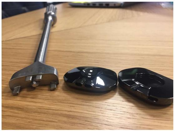
The tool is designed in a such a way that it is not possible to use it with 2 identical plates.
