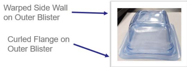
Image 1: Example of damaged packaging
