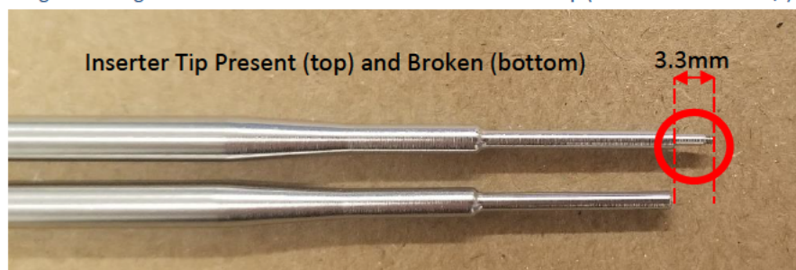
Figure 1. Surgical-Grade Stainless Steel Inserter and Inserter Tip (3.3mm L x 0.97mm \varnothing )
