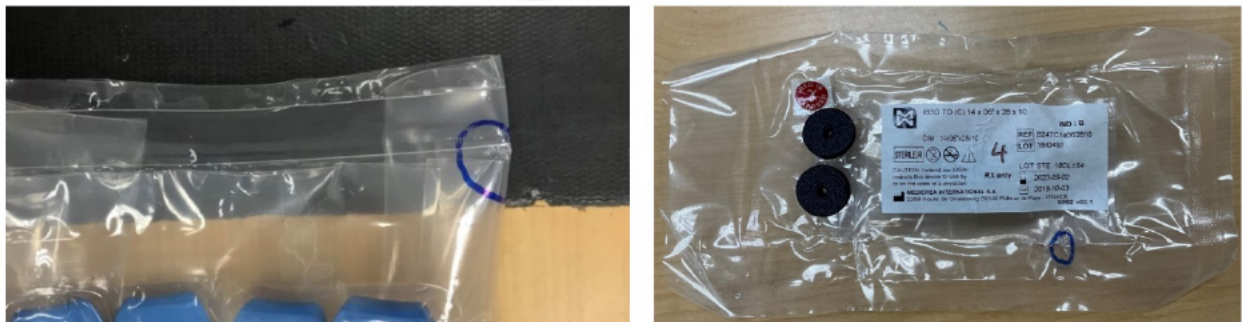
Figure1: Photos of pinhole leaks identified in sterile barrier (circled in marker)
