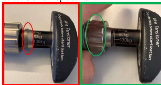
Left: Incorrect position of adjustment ring; Right: Correct position of adjustment ring
