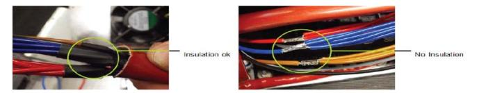
The Monitor and/or the IO Tablet may lose power if non-insulated wires come into contact with each other.
