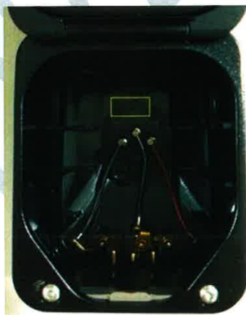
Photo 2: Lot Number is located inside the housing. The yellow box does not exist on the product. It has been added to the photo to identify the location.
