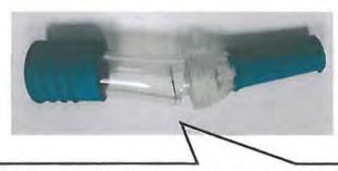
LEAKAGE: the 3/8" PVC tube was not properly glued
