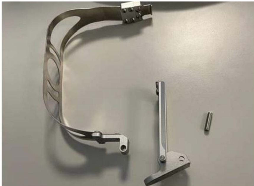
Picture 3 Disassembly of the Transport Guard due to loosened cylindrical pin.
