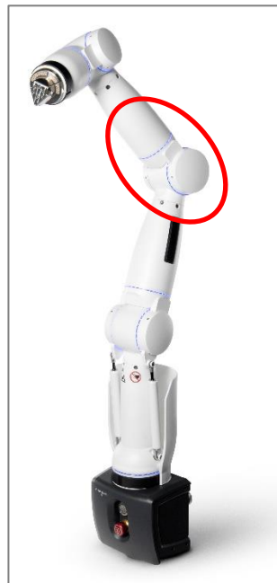
Picture 1 – Cirq Arm System 2.0 with the area around joint 4 marked, where potentially affected screws were used
