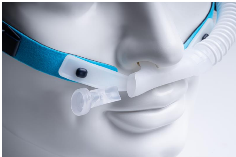
Figure 1: An In2Flow Nasal cannula size M is shown. The plug became detached from the opposite side of the tubing. (This is an example; sizes S and L are also affected.)
