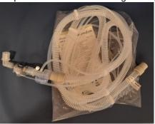
Step 3: Detach the elbow from the breathing circuit and discard it.
