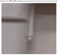
Not conform: Crack in intellipack packaging tray
