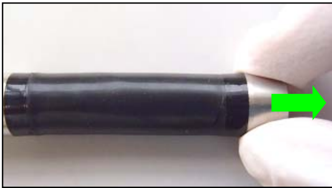
Cut Sample 2: Cuts can be easily detected by pulling.
