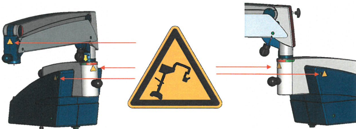
Figure D: Position of new Warning Label
