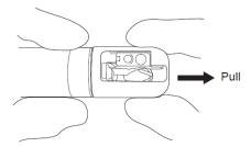
**6** Twist the distal cover gently in both directions and confirm that the distal cover on the distal end of the endoscope does not slip and come off.
