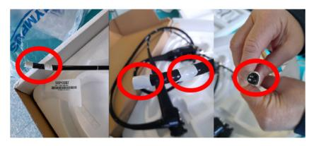
This white tape is used during the repair process to protect sensitive parts of the endoscope from damage, (scratches and dents). It is to be removed during final
