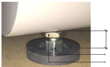
Max. 20 mm between the top of the height adjuster and the round pipe
