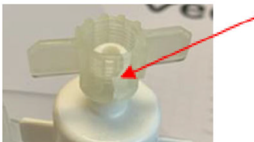
Figure 2: Example of a cracked adaptor
