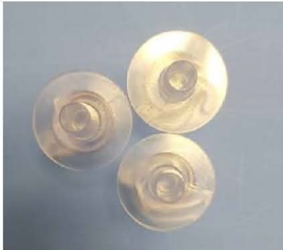
Picture 1 – Incorrect filter connectors with occluding fleece.
