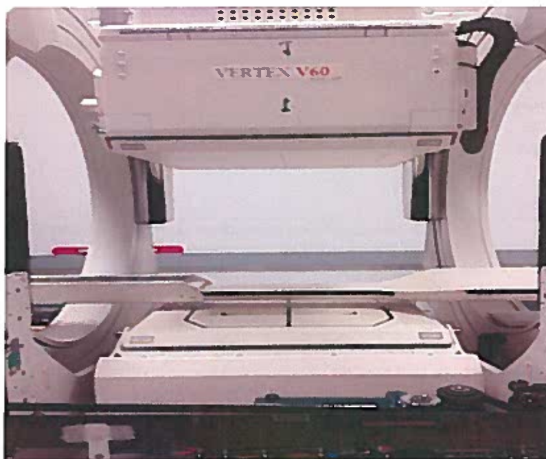
Picture 2: Lateral view of the Superior/Inferior Detector heads
