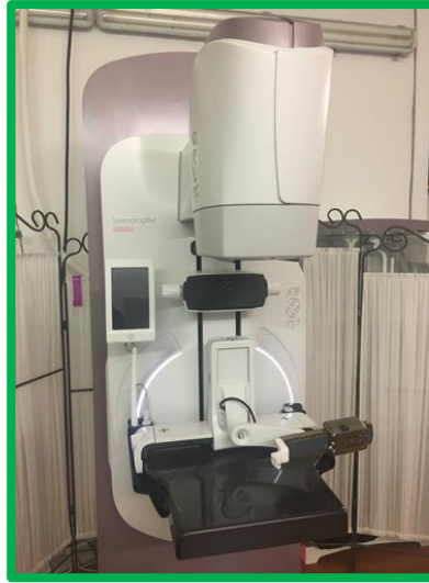
Figure #2 – Acceptable Gantry Position for Biopsy Procedure: Senographe Pristina gantry rotation angle is 0°. Horizontal approach setup.
