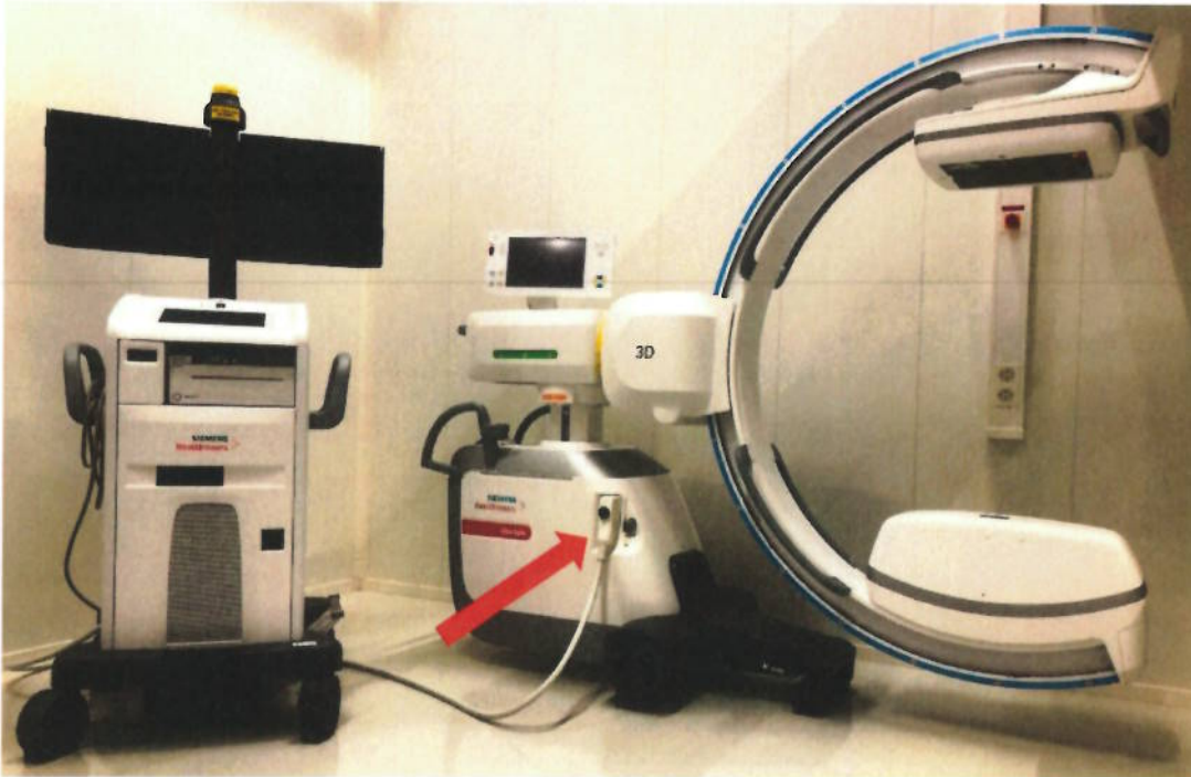
figure 1: example of monitor trolley connected to the X10 connector of the main unit (c-arm) by main cable
