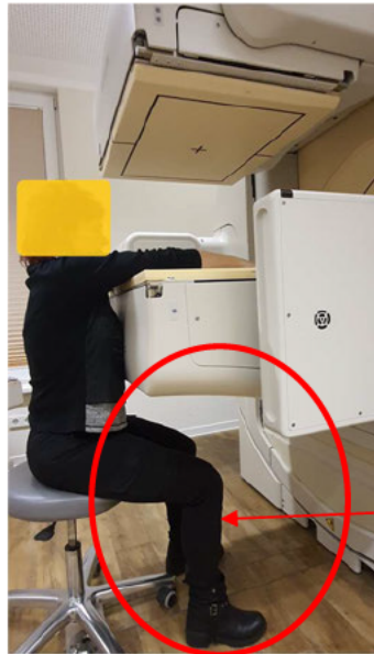
Figure 3. Avoid positioning a patient's lower limbs under the detector below Center of Gantry
