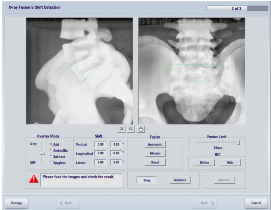
Figure 1: X-Ray Fusion – bony fusion to DRR to determine the shift to desired patient position.
