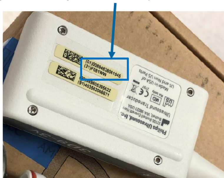
Figure 3 Device Identifier and Serial Number printed on the Connector.
