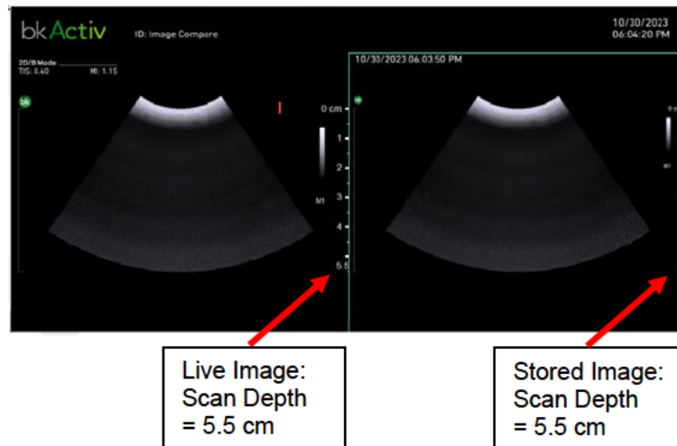
Figure 1. bkActiv screen during Dual Live Compare. Same scanning depth is used on Live image (left panel) and Stored image (right panel)
